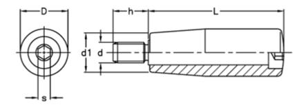
$$\begin{array}{ll} D & = 18 \\ d1 & = 15 \\ d \ 6g = M6 \\ h & = 13 \\ L & = 40 \\ s & = 4 \end{array}$$
